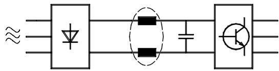
The voltage distortion on the mains supply depends on the size of the harmonic currents multiplied by the mains impedance for the frequency in question. The total voltage distortion THD is calculated on the basis of the individual voltage harmonics using the following formula:
