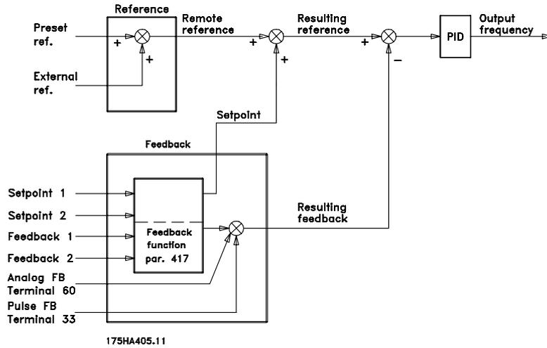
As can be seen, the remote reference is totalled with setpoint 1 or setpoint 2. See also *Reference handling*. Which setpoint is to be totalled with the
