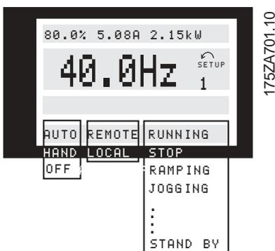
The left part of the status line indicates the control element of the frequency converter that is active. AUTO means that control is via the control terminals, while HAND indicates that control is via the local keys on the control unit.
