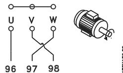
The factory setting is for clockwise rotation with the VLT frequency transformer output connected as follows.
