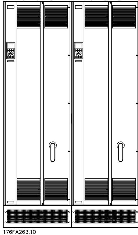
All units in the above-mentioned series require a minimum space of 225 mm (8.9 in) above the enclosure and must be installed on a plane floor. This applies to IP 21/NEMA 1 and IP 54/NEMA 12 units. Gaining access requires a minimum space of 579 mm (22.8 in) in front of the frequency converter.
