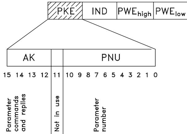
Parameter commands and replies (AK) Bits no. 12-15 are used for transferring parameter commands from master to slave and the slave's processed reply back to the master.
