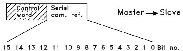
The serial communication reference is transmitted to the frequency converter in the form of a 16-bit word. The value is transmitted as whole numbers 0 - ±32767 (±200 %). 16384 (4000 Hex) corresponds to 100 %.
