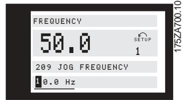
The chosen digit flashes. The bottom display line shows the data value that will be entered (saved) when signing off with [OK].
