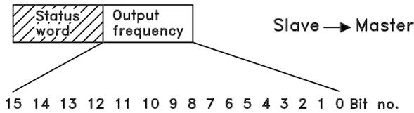
The value of the present output frequency of the frequency converter at any given time is transmitted as a 16-bit word. The value is transmitted in the form of whole numbers 0 -± 32767 (±200 %). 16384 (4000 Hex) corresponds to 100 %.
