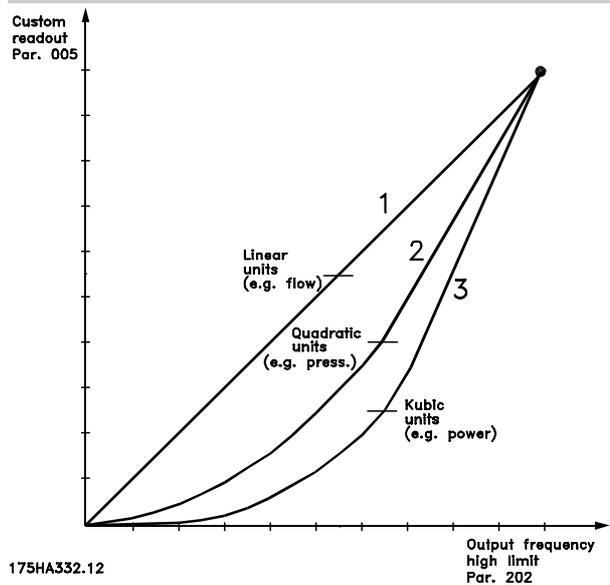
Select a unit to be shown in the display in connection with parameter 005 *Max. value of user-defined readout*. If units such as flow or speed units are selected, the ratio between readout and output frequency will be a linear one.
