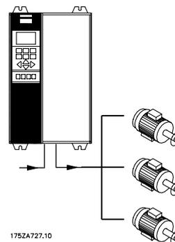
VLT 8000 AQUA is able to control several motors connected in parallel. If the motors are to have different rpm values, the motors must have different rated rpm values. Motor rpm is changed simultaneously, which means that the ratio between the rated rpm values is maintained across the range.
